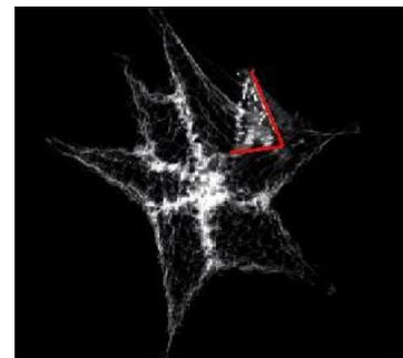
*Figure 1 RemoveDEBRIS net deployment, with the target satellite highlighted (Source: RemoveDEBRIS team)*
